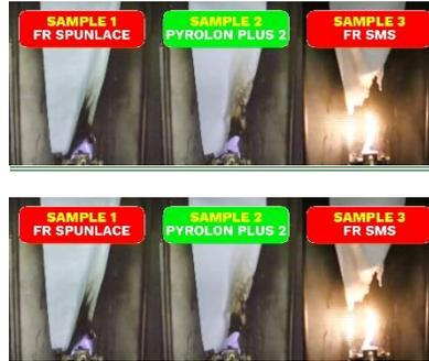
A video, showing the relative performance of different SFR fabrics when contaminated with a light oil, can be viewed [here](#).
